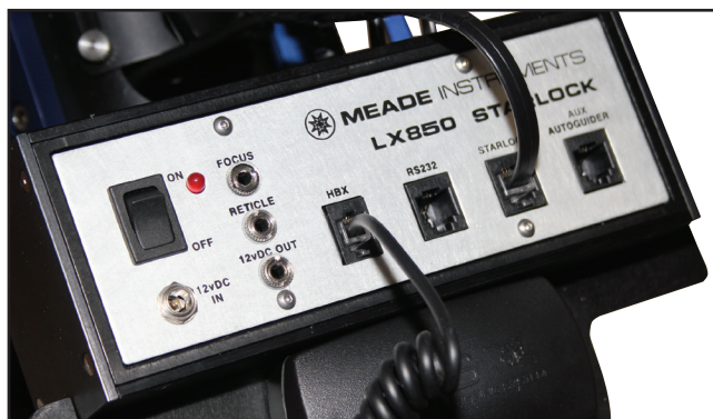
Fig 27: Connect handbox cable to HBX
