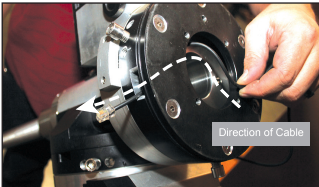
Fig 17: Routing cable under the saddle plate.
