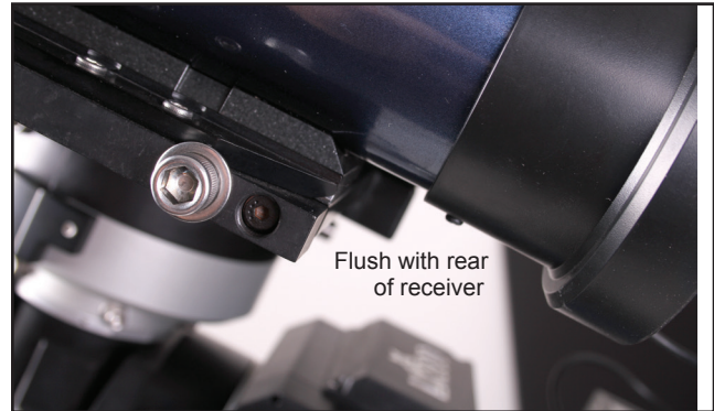
Fig 45: Position StarLock flush with the receiver.
