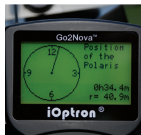
A robust screw ( left ) provides precise adjustment of the polar-axis altitude. The hand controller's 8-line display ( right ) also shows the location of Polaris on the polar-alignment reticle when the mount is properly aligned ( below ).
