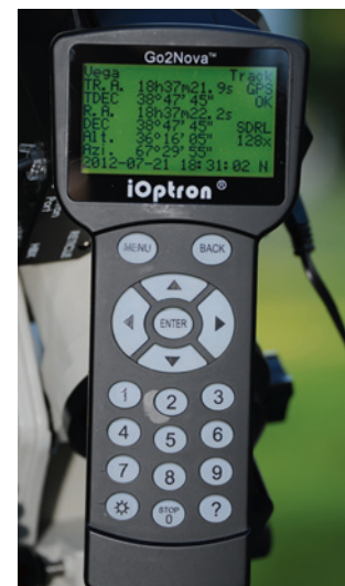
A robust screw ( left ) provides precise adjustment of the polar-axis altitude. The hand controller's 8-line display ( right ) also shows the location of Polaris on the polar-alignment reticle when the mount is properly aligned ( below ).
