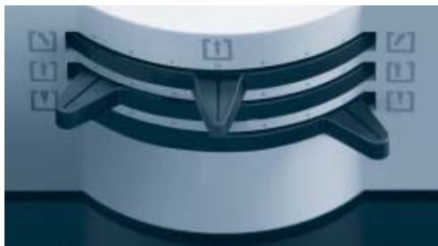
Setting: Brightfield for transparent, high contrast specimens and also used to display contours and outlines
