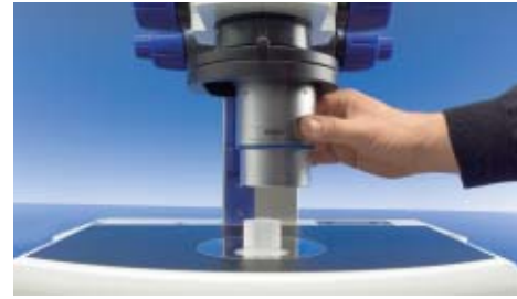
Simple switching from stereoscopic observation to a parallax free macro view of the object by the camera
