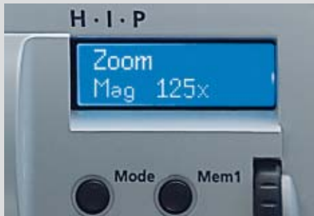
The wheel responds dynamically to the movement of the thumb: slowly and sensitively with small movements and more quickly with larger movements.
