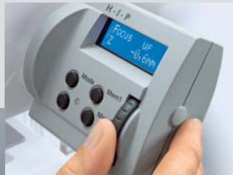
The wheel responds dynamically to the movement of the thumb: slowly and sensitively with small movements and more quickly with larger movements.
