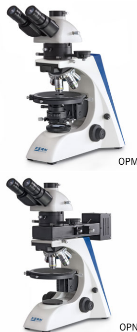
Bertrand lens, \lambda Slip, 360° rotatable analyser (removable)
